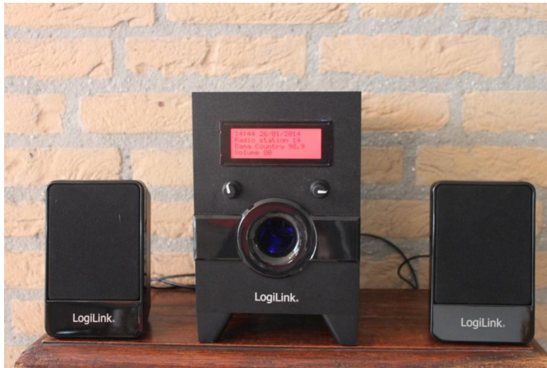
Figure 5 Raspberry PI internet radio with Rotary Encoders
